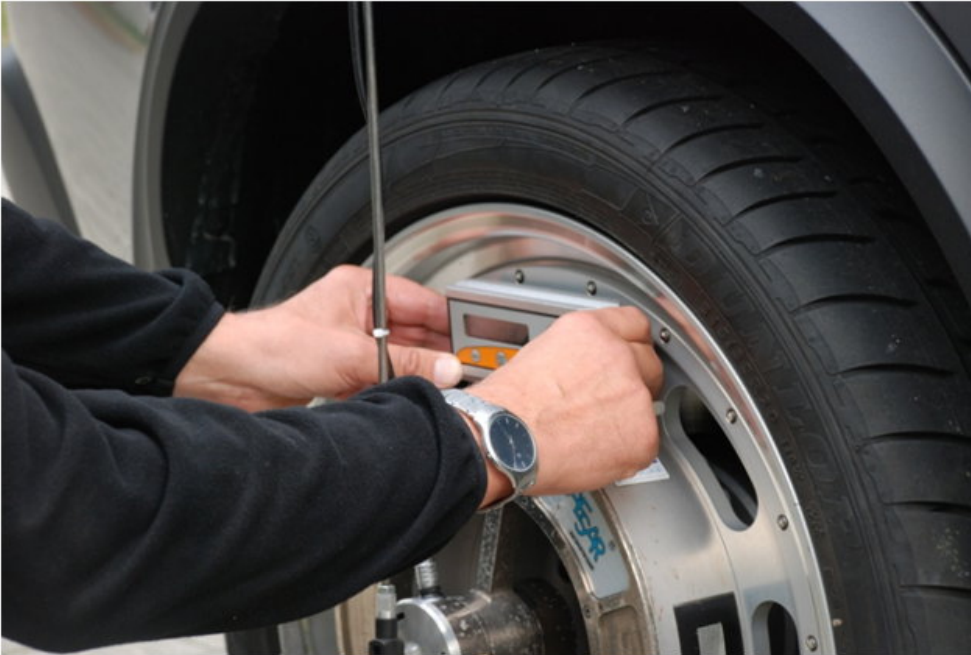
Fig. 28: Measuring with the bubble level
