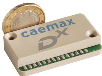
Signal conditioning and transmitter unit (SCT)
