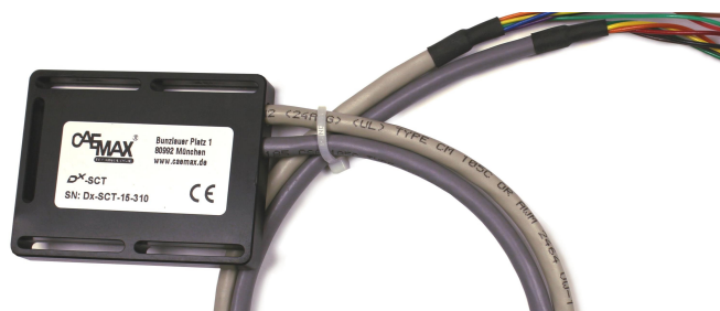
Signal conditioning and transmitter unit (SCT) in IP67 housing
